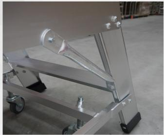
**STEP SIX** Firmly Tighten all nuts and bolts from earlier steps
